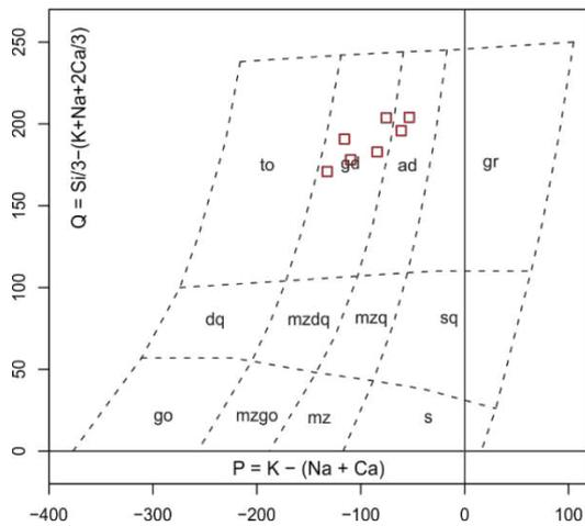
Fig. 9-4 Classification of the Bíteš Gneiss in diagram of Debon – Le Fort (1983) .
