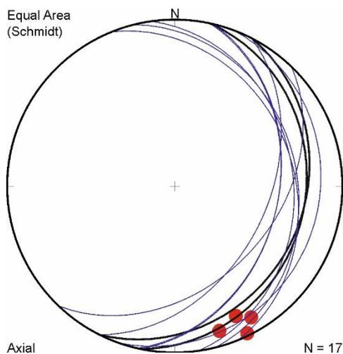
Fig. 12-2 Orientation of structures at the locality: navy blue great circles – foliation, red dots – stretching lineation; thick black great circles – rock boundary.
