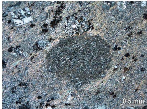
Fig. 1-2 Texture of rhyolite metatuff with chess board albite and oval basalt fragment, XPL.
