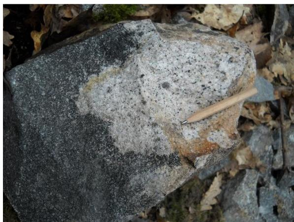
Fig. 8-2 Cauliflower texture at contact of biotite–amphibole diorite and biotite granite.
