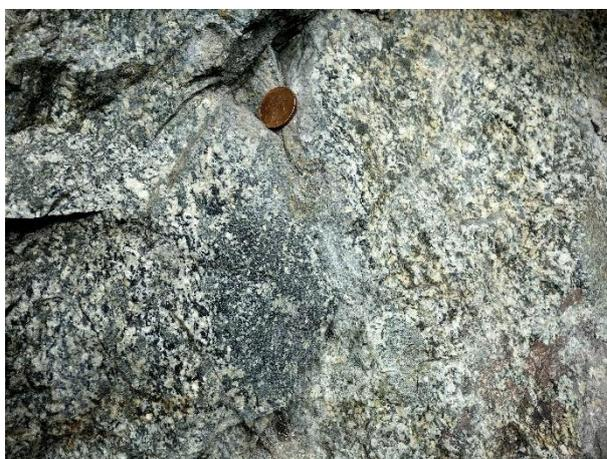
Fig. 2-3 Altered diorite with mafic enclave. Steep foliation, alteration and cataclasis effects are visible.
