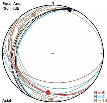
Fig. 3-6 Orientation of foliation (great circles) and lineation (dots): red – Svatka Massif; blue – Devonian limestone; brown – Bílý potok Group. Fault surfaces by black colour.
